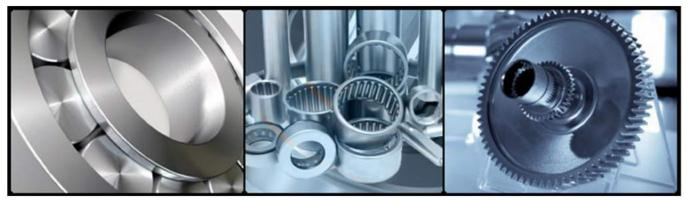
"Armoloy TDC™ (Thin Dense Chrome) is a hard (78 Rc), thin, dense chromium coating with a micronodular surface texture. The coating's nodular finish reduces the amount of surface area exposed to surfaces in contact with it, thereby substantially reducing friction and extending wear life. This nodular finish also retains smaller amounts of industrial lubricants for longer periods, both further reducing friction and creating a cleaner work environment."
